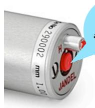
Probe pressure adjustment screw The cylindrical probe has an adjustable load in one of three ranges.
