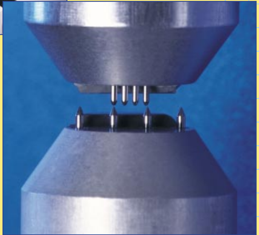
Contrast between our smallest and largest spacing probe heads 0.500 and 1.591mm (shown approx x 10)
